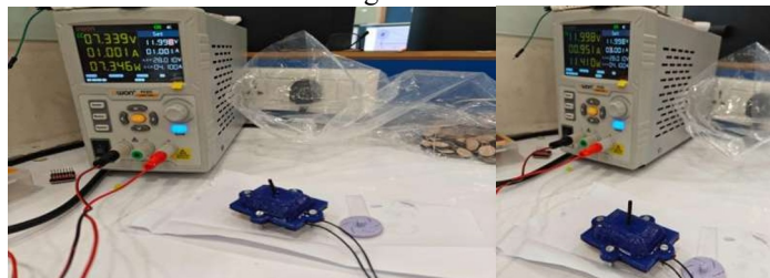
Fig. 9: (a) Pin fell down due to cold expansion media and (b) Pin upright due to sufficient voltage to PTC heater expanding the silicone oil media.
