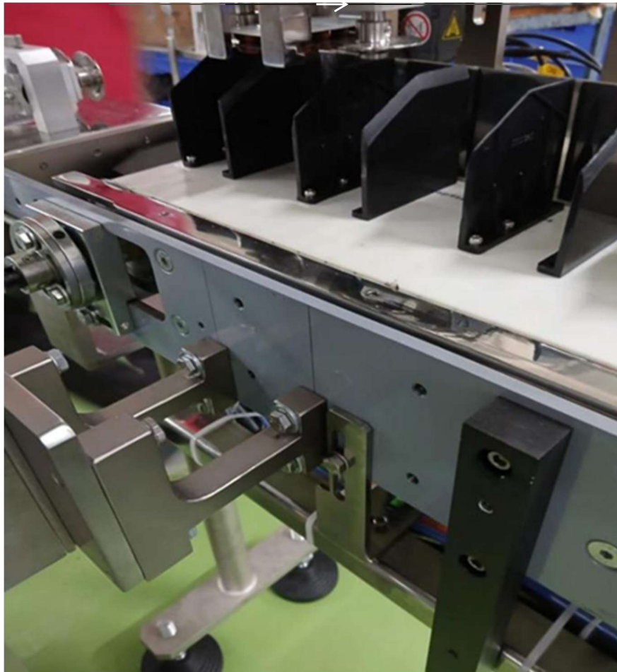
Fig. 1 Mounting plate fitted in a typical conveyor system
