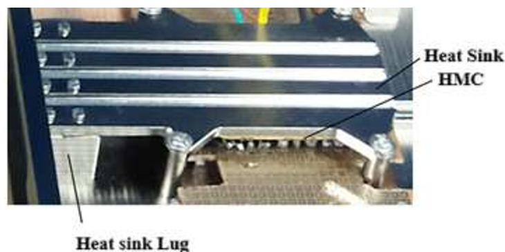
Fig. 6. Fabricated heat sink attached on heat source
