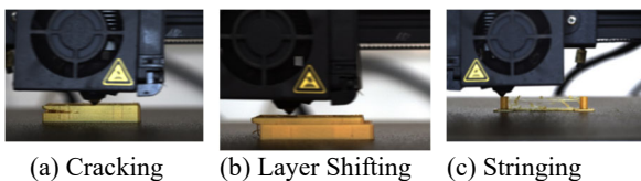
Fig. 3 3D printing defects
