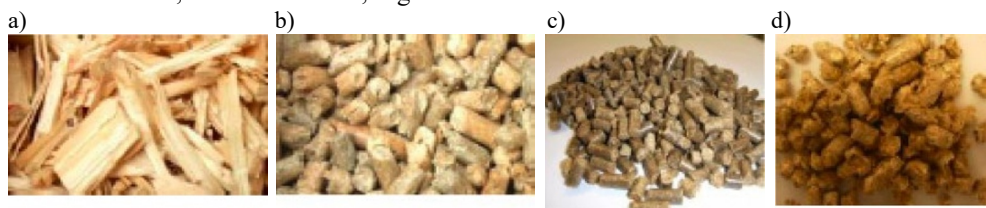
Fig. 1. The types of renewable fuels utilized for gasification process to obtain low calorific gas fuel: a) wood chips, b) wood pellets, c) straw pellets, d) miscanthus pellets.
