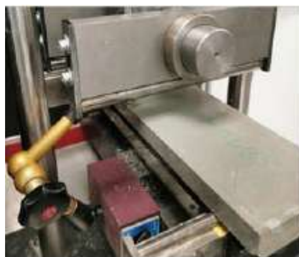
Fig. 8. Sample during 4-point flexural test
