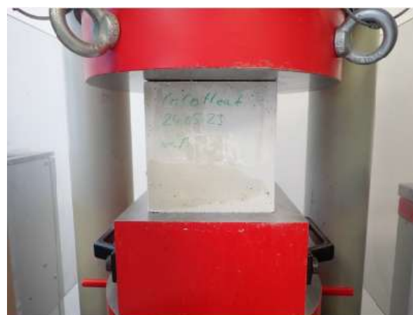
Fig. 9. Sample during compressive test
