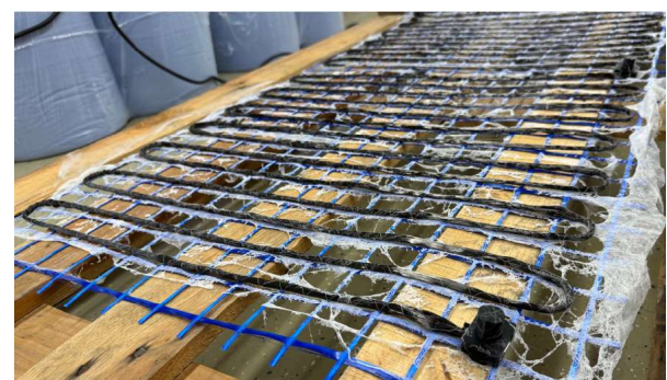
Fig. 5. Carbon roving molten onto fiber reinforcement
