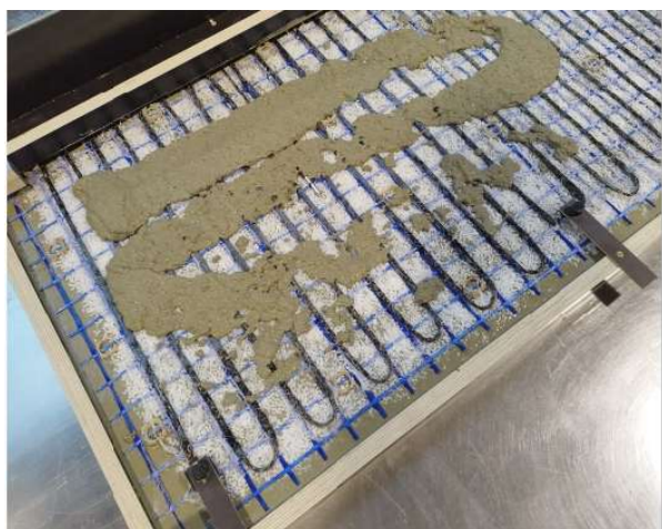
Fig. 6. Casting process with mold, carbon roving, textile, PCM, sensor and concrete
