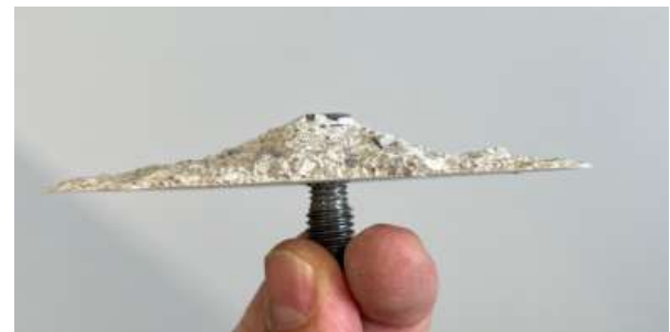
Fig. 17. Cone-shaped concrete body with thread adapter
