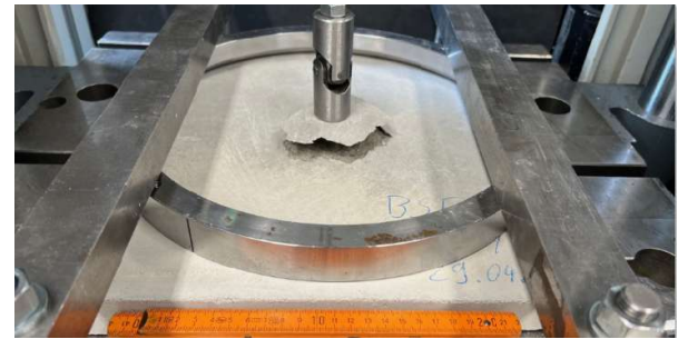
Fig. 16. Completed Pull-out test
