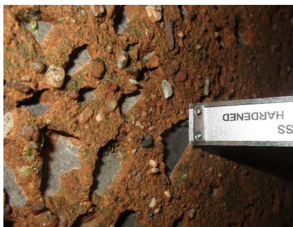
Fig. 3. Dissolution of highly porous coarse calcareous aggregate and no effect on fine siliceous aggregate.
