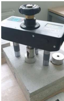
Fig. 2. Measurement of bond strength by the pull-off test method.
