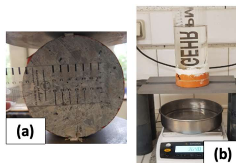
Fig. 1. Crack width controlled with a ruler during the splitting test (a), Water Permeability test (b).
