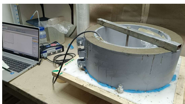
Figure 1. Specimen arrangement for the restrained ring test.
