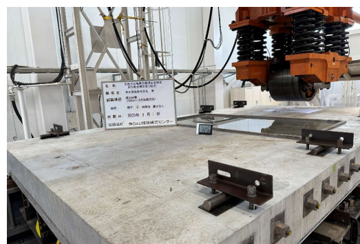
Fig. 11. Testing status (water leakage test at STEP-1)
