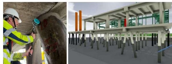
Fig. 15. Execution of potential mapping via one-wheel-electrode ( CuCuSO_4 ) + schematic overview of the jetty.
