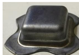
Fig. 14. Formed cup in square cup drawing and ironing process (C10)
