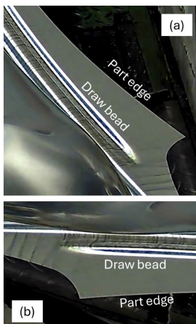
Fig. 2. (a) Raw image captured at the location of balance blocks 2 and 3 and (b) the corresponding image after perspective correction. In both images, the formed part appears in light grey, with the draw bead locations highlighted by overexposed white regions, while the surrounding area remains dark.
