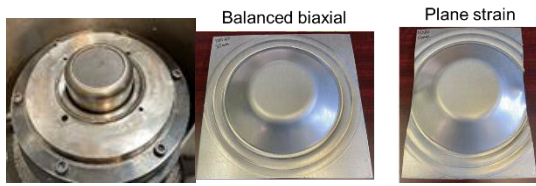
Fig. 5. Marcink tooling and prestrained samples for biaxial and plane strain conditions
