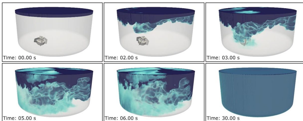
Figure 6. Fluid tracing in the existing vessel
