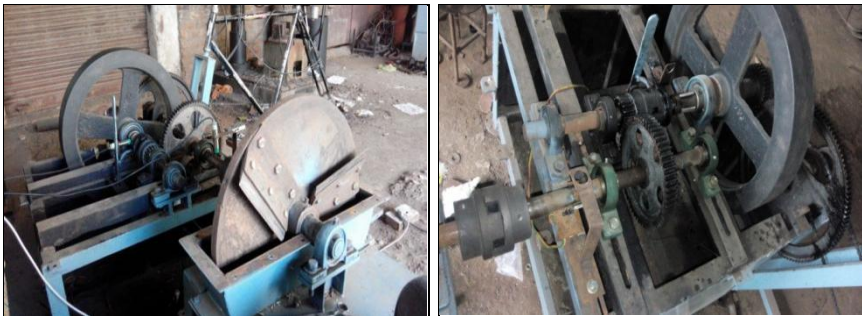
Fig. 1. Innovative arrangement of man operated Propeller Device including Wood Chipping Unit.
