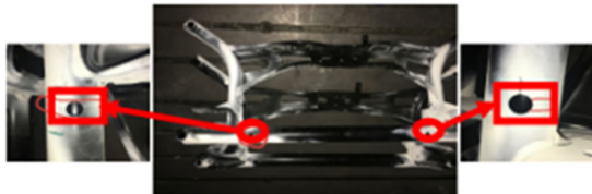
Fig. 10. Cracked left and right process leakage holes [15]
