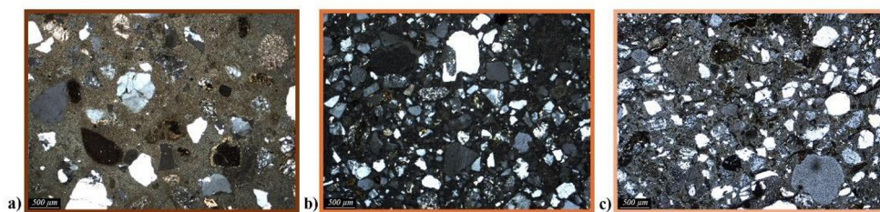
Fig. 5. Frame of thin section: image under PLM, xpl. a) Bedding mortar of Brunelleschi's Dome of the Florence Cathedral; b) Bedding mortar of Tornabuoni Chapel of Santa Maria Novella's church; c) Bedding mortar of Davanzati Palace.
