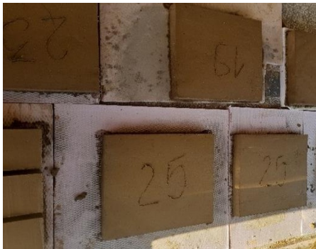
Fig. 6. Samples of bricks after pulling from the moulds
