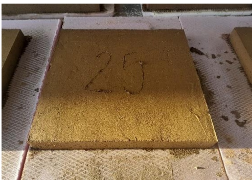
Fig. 6. Samples of bricks after pulling from the moulds
