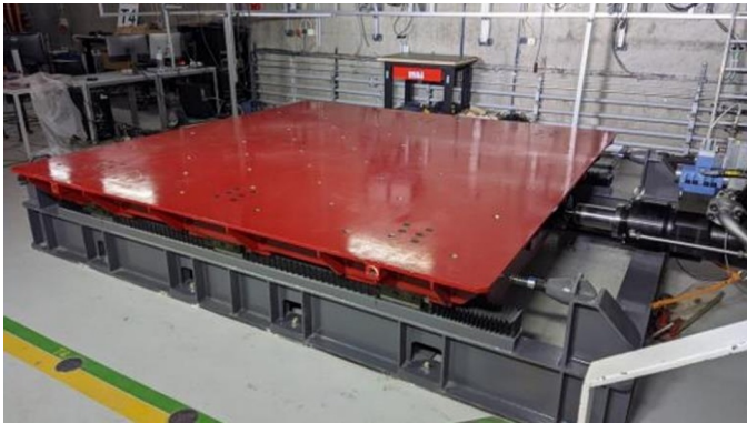
Fig. 3. View of the shaking table facility.
