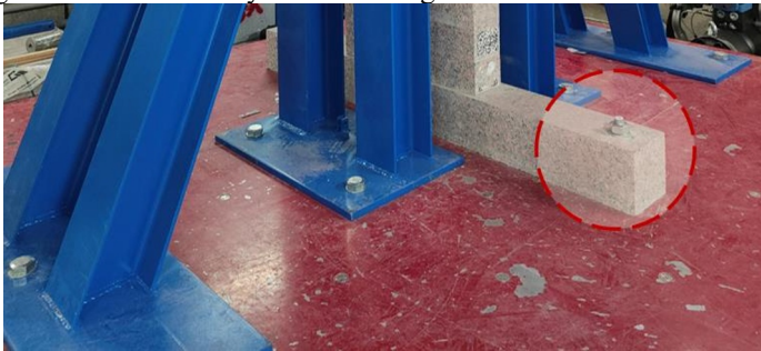
Fig. 4. The VSSW setup: close view of the base boundary condition. The red-dashed circle highlights the connection between the base block and the shaking table.
