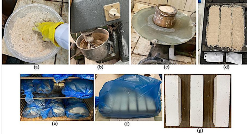
Fig. 1. (a) Preliminary mixing of raw materials; (b) Producing mortar through a mortar mixing machine; (c) Arrangement of water quantity by flow table test; (d) Molding of the fresh mortar; (e) Curing of mortar in the oven; (f) Storing of the specimens after oven curing; (g) The specimens that were ready for the tests.
