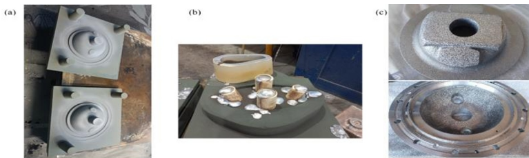
Fig.7. a) Printed sand mold by BJ method, b) Casting process of aluminium spare part, and c) part after casting and machining
