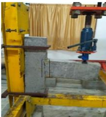
Fig. 7. Cracks observed in specimen with 150mm stirrups spacing.
