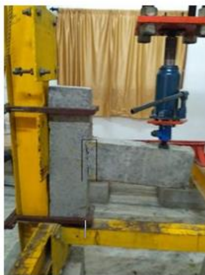
Fig. 6. Cracks observed in specimen with 70mm stirrups spacing.
