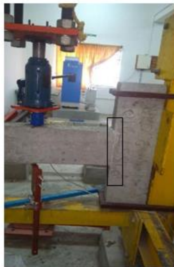
Fig. 5. Cracks observed in specimen with Stirrups spacing -100 mm.
