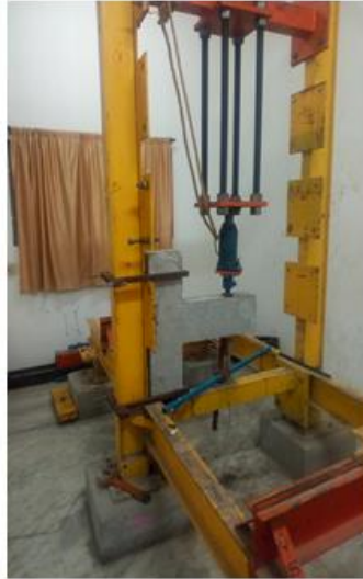
Fig. 4. Loading frame and Hydraulic jack attached to specimen.
