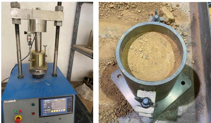
Fig. 4. Equipment for CBR test and soil sample
