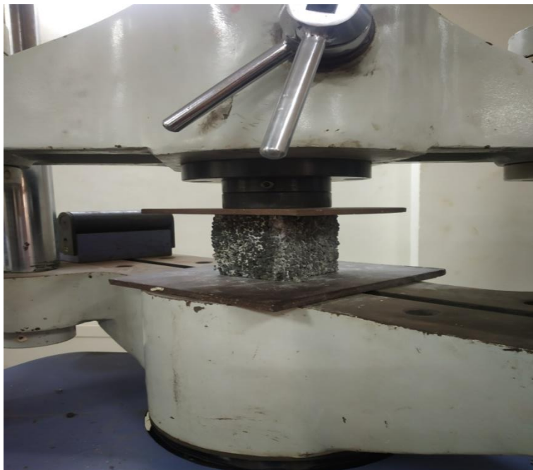
Fig. 8. Compressive strength test
