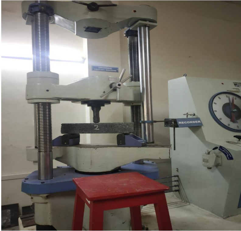
Fig. 12. Flexural strength test
