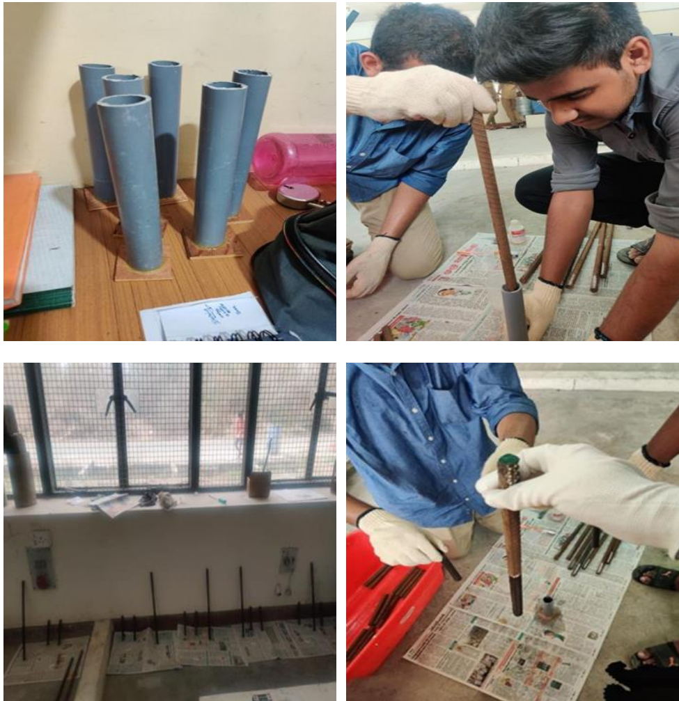
Figure 2 Coating of the rod with Zirconium Epoxy
