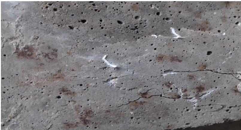
Fig. 9. Self-healing of bacterial concrete (75 ml solution) of M25
