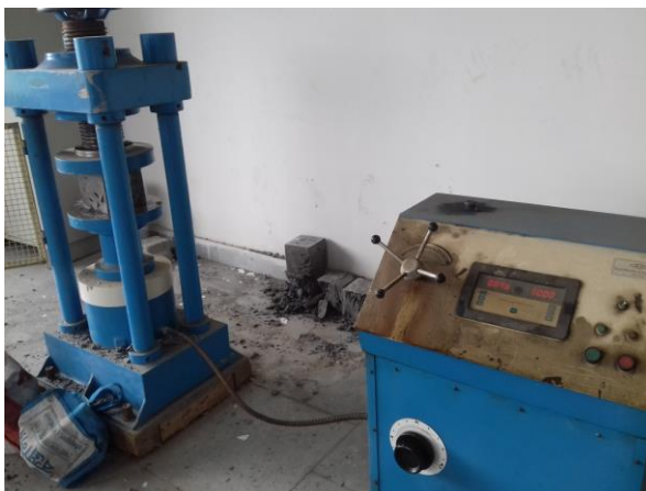
Fig. 3. Cubes under compression test
