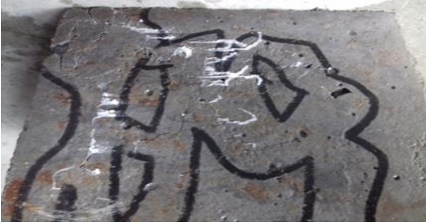
Fig. 10. Self-healing of bacterial concrete (90 ml solution) of M25
