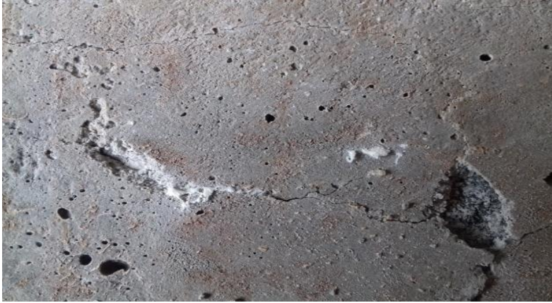
Fig. 8. Self-healing of bacterial concrete (60 ml solution) of M25
