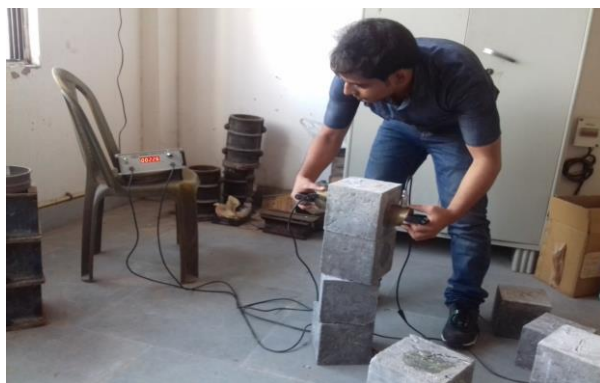
Fig. 4. Ultrasonic pulse velocity test
