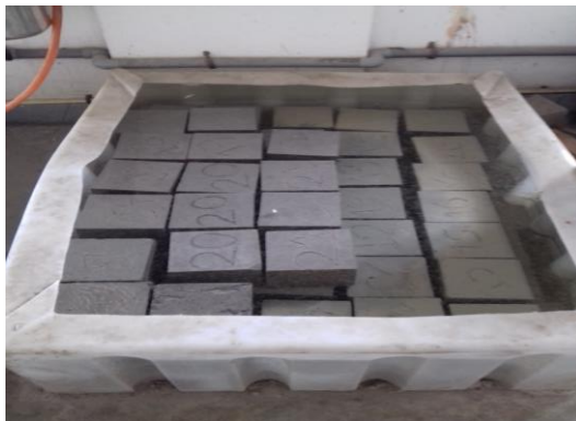
Fig. 2. Concrete cubes under curing
