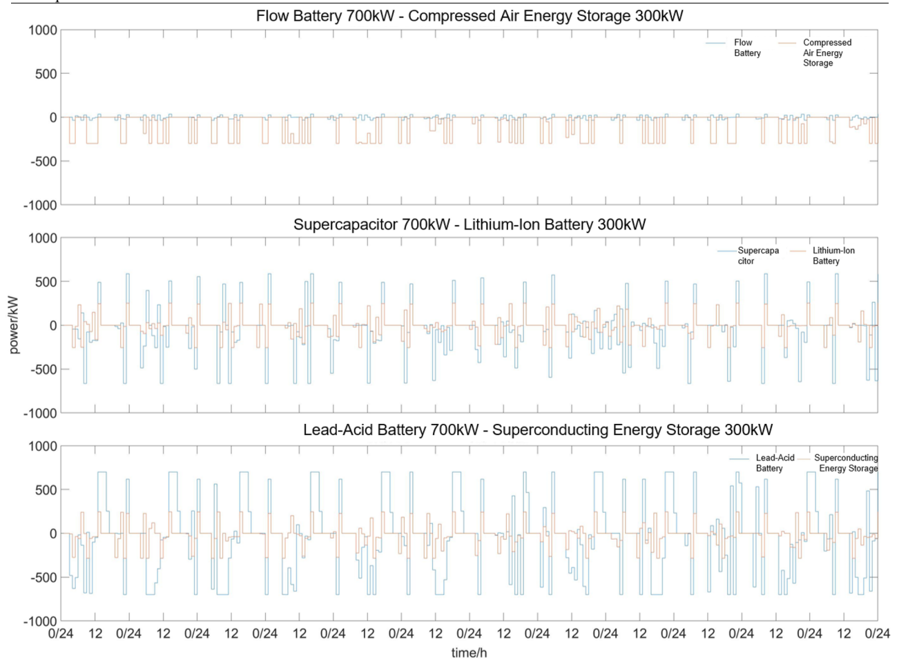
Fig. 7. Charge and discharge power of hybrid energy storage battery at each time node
