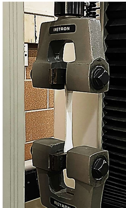
Figure 3: Tensile Testing using Instron Tensile Testing Machine
