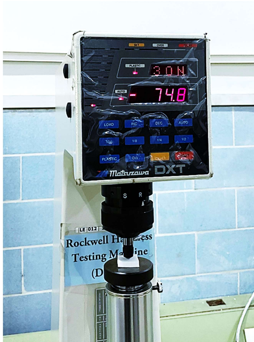
Figure 4: Hardness Testing using Rockwell Hardness Testing Machine
