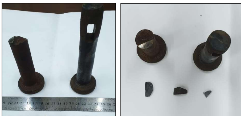
Figure 3: Damaged hanger and new hanger along with pins and their samples
