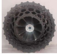
Figure 7 Developed wheel for Throwable Unmanned Ground Vehicle
