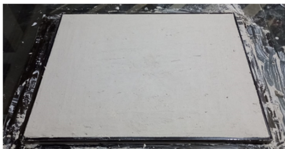
Fig. 11. Carلودuvica Palmata reinforced gypsum composite panel
