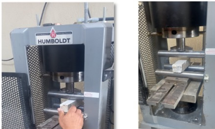
Fig. 3. Flexure testing process
