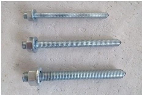
Fig. 9. Steel threaded rods of M8, M10 and M12 bonded anchors.
