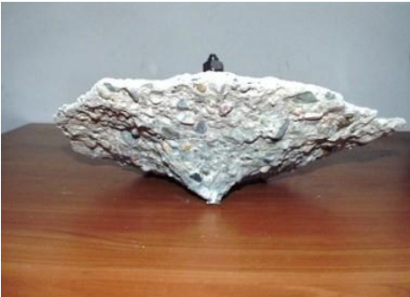
Fig. 3. Destruction of the connection made observed in the tests expansion anchors.
