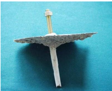
Fig. 5. Characteristic failure mode for bonded anchors.
