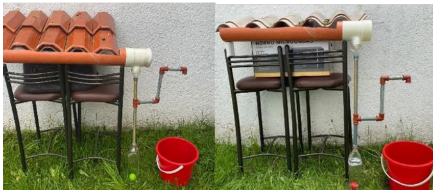
Fig. 1. Left: asbestos cement roof; right: tile roof.
