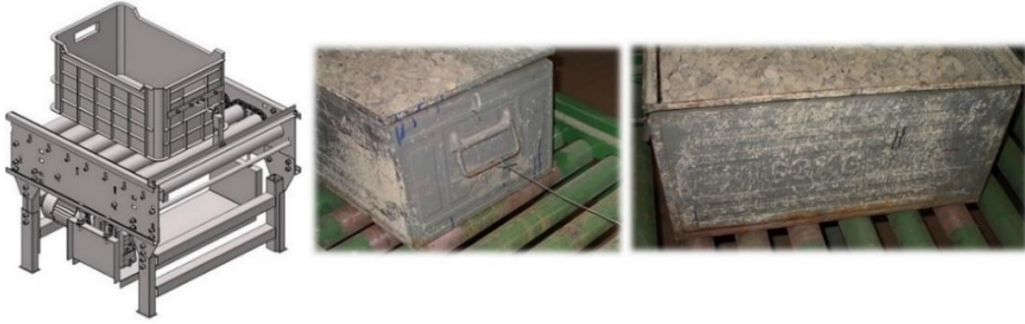
Fig. 5. Positioning the storage crate on the roller track rollers.
