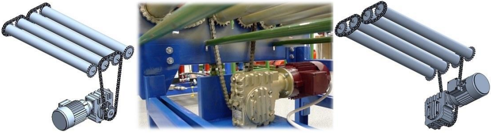
Fig. 3. Transfer of traction force from the drive to the rollers of the roller conveyor.
