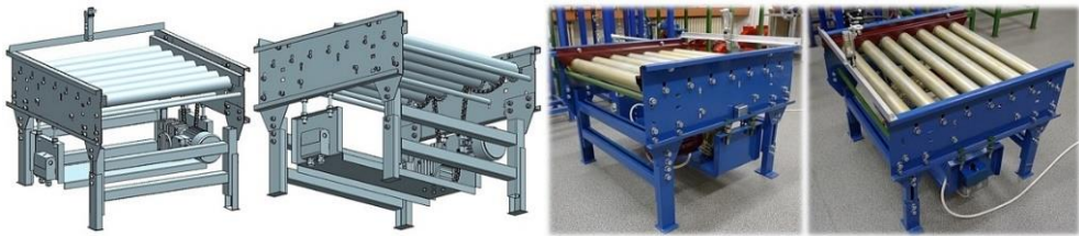
Fig. 1. Experimental device - powered roller conveyor a) 3D model created in SolidWorks, b) implemented roller conveyor.
