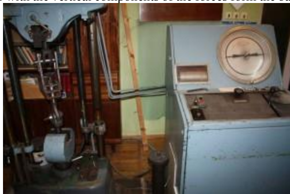
Fig. 1. Equipment for testing coupling devices with load application in horizontal and vertical directions [3].
