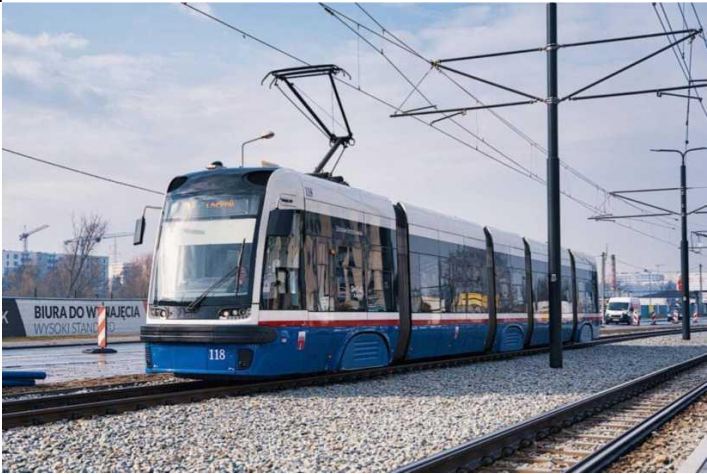
Fig. 3. Tram equipped with a power supply system from the overhead contact line [1].
