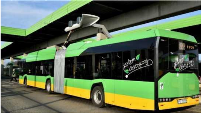
Fig. 2. Charging an electric bus with a stationary pantograph charger [20].
