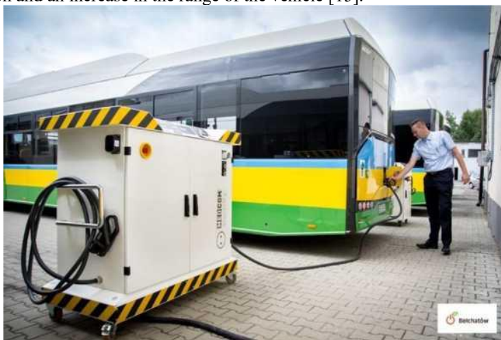
Fig. 1. Charging an electric bus with a plug-in plug [18].
