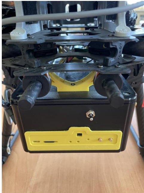
Fig.5. The authorial prototype of the measurement system, mounted on UAV.
