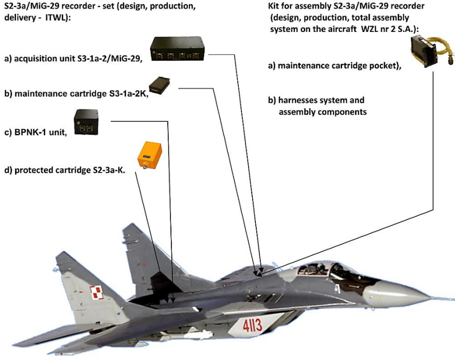
Fig. 3. Assembly of the S2-3a recorder on MiG-29 aircraft.
