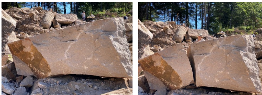
Fig. 3. Splitting of a boulder with one charge of 50 g Mixture #2 in single blasthole with length 0,60 m.
