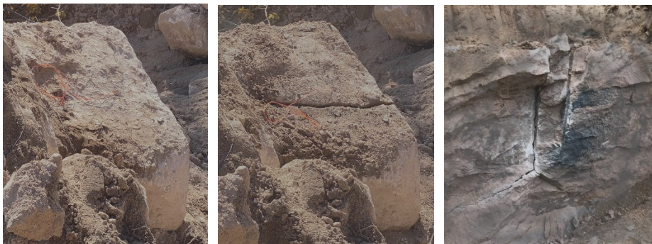
Fig. 4. Splitting of rock body with two parallel boreholes. Effects from preloaded bottom charge of 300 g. Mixture #3 and decked second charge of 150 g. Mixture #3 in every single blasthole with length 1,80 m.
