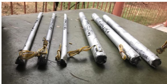
Fig. 1. Test samples - loaded and plugged aluminium pipes with electric igniter
