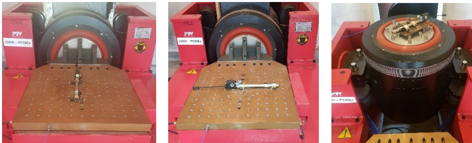
Fig. 9. Fixation of seatbelt pretensioner in view of exposure to vibrations on the X, Y, Z axes
