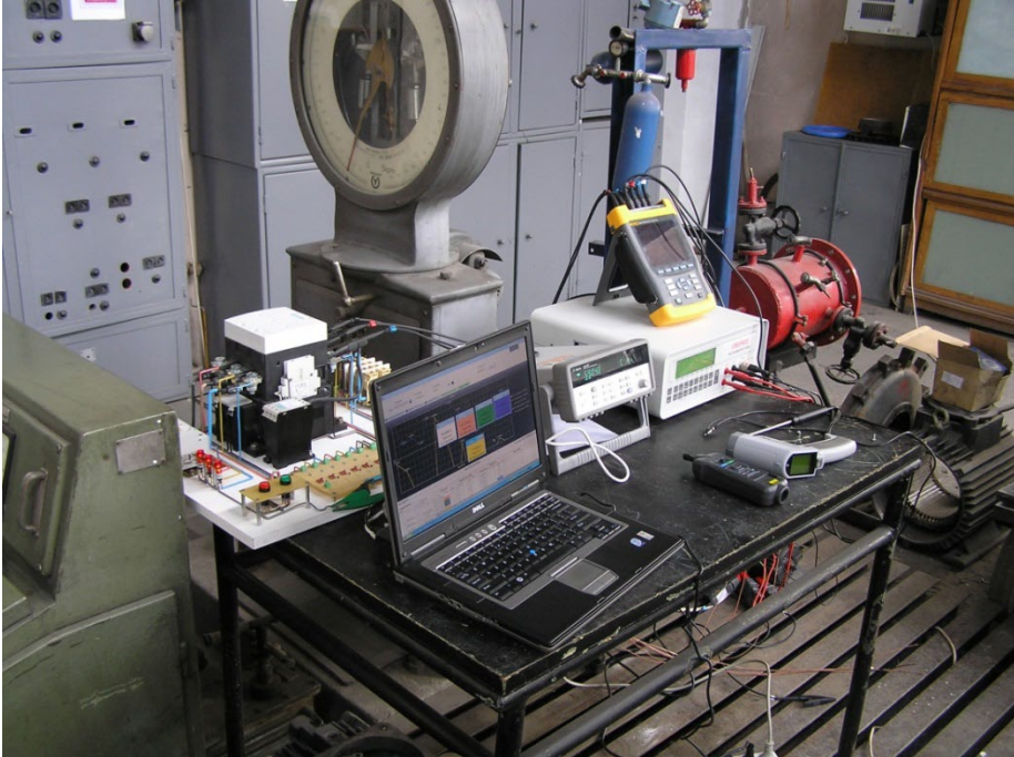
Fig. 1. Test stand for determining the maximum surface temperature of electric motors
