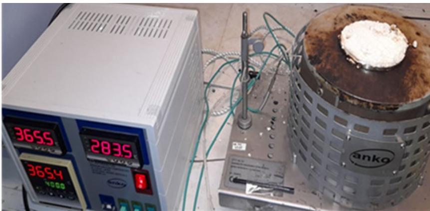
Fig. 2. Stand for determining the minimum ignition temperature of the dust cloud
