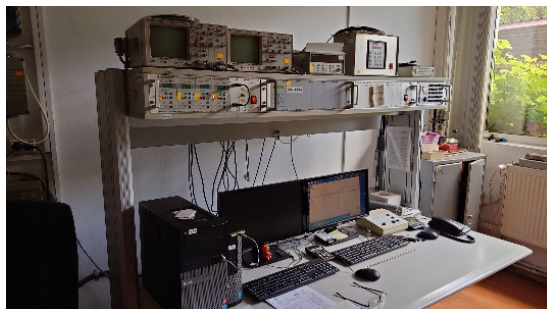
Fig. 3 Command and control of the test rig to perform tests in explosive mixtures
