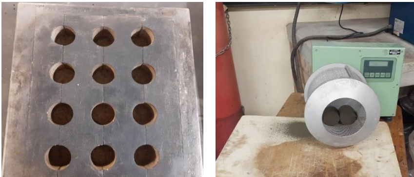
Fig. 3. Friability patterns with friability tester on the right
