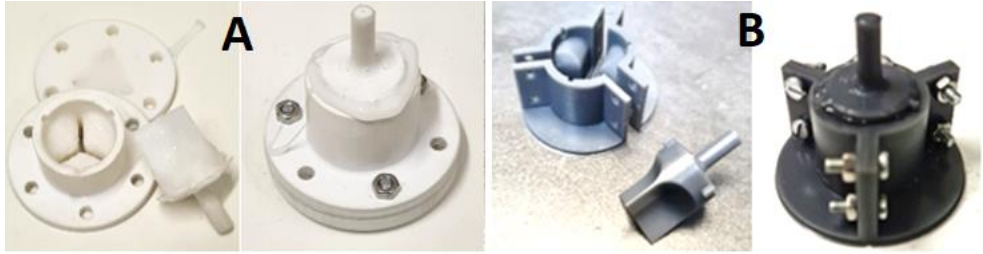
Fig. 2.1. Design configuration A (White resin (Rigid 10K)) and B (Grey resin (Tough 2000)).
