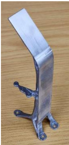
Fig. 6. Printed part in AlSi10Mg.
