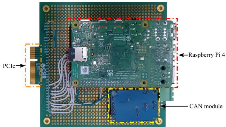
Fig 5: CPU with PI4 and CAN module on PCIe plugin card
