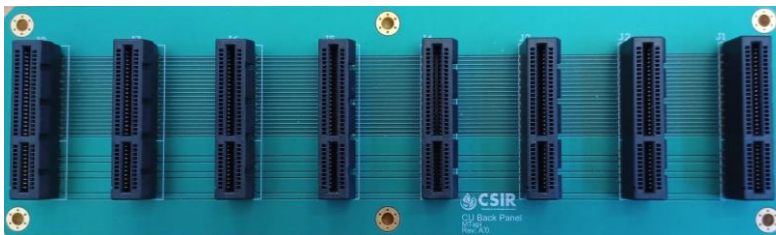
Fig 6: Control Unit backplane using PCIe connectors.
