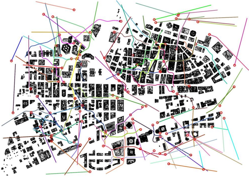
Fig. 18. Snapshot taken 50 s into one of the Monte Carlo simulations in the 50-60 m altitude range. The current position of each UAV is circled in red with its trajectory up to that position also shown.
