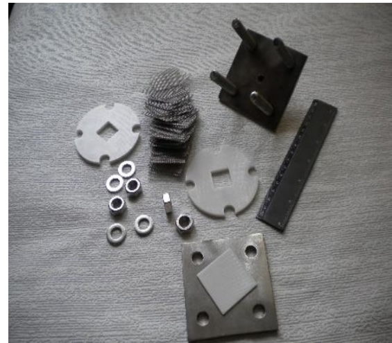
Fig. 3. Exploded rigging and original woven meshes.
