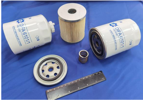
Fig. 1. Filter DIFA 6101/1 assembled and disassembled.
